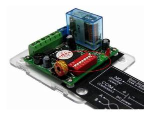
This device is to be physically installed inside the premises, and it is connected to the iGuard's *Remote Relay* connector at the back of the unit through a special twisted-pair cable.
