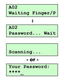
3. If the Fingerprint or the Personal Password matches the record, the user will be authenticated, and the unit will return to the Standby Mode.
